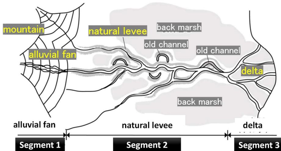
[Figure 3] Segments and the topography around the river <sup>(c)</sup>
