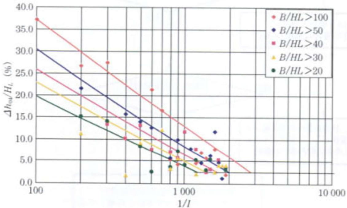
[Figure A.2] Water level rise due to sandbar formation (reference based on past experience) ( $H_t$ ,  $B$  are the water depth and river width at the time of the average annual maximum discharge, respectively, and  $I$  is the riverbed slope)
