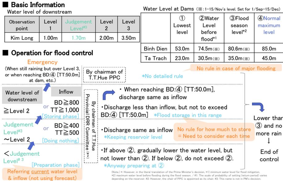
(a) Flood control operation at Binh Dien Dam (Huu Trach River) and Ta Trach Dam (Ta Trach River)
