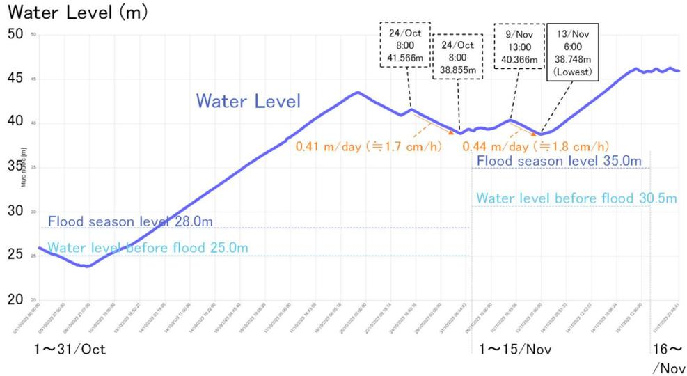
[Figure 7] Reservoir water level in TT from October to the November flood
