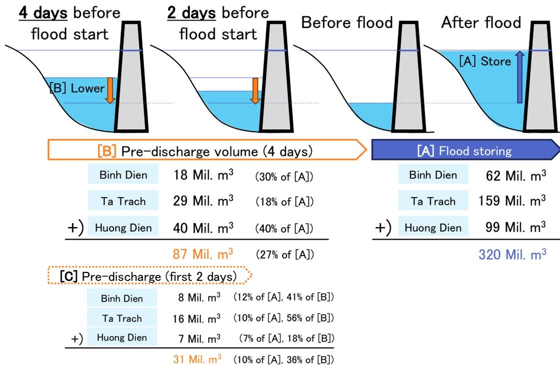
[Figure 8] Stored water volume [A], the capacity secured by the prior lowering reservoir water level [B], and the capacity secured during "first 2 days" of the 4-day period of lowering reservoir water level [C] in the three major dams (Data source: same as Figure 6)
