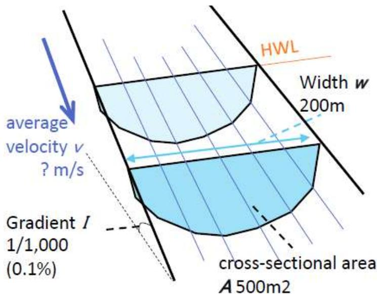
[Figure 6] Example of river channel for calculation of discharge
