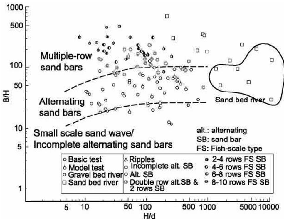
[Figure 9] Appearance of sandbars depends on the river width-depth ratio (B/H) <sup>(d)</sup>
