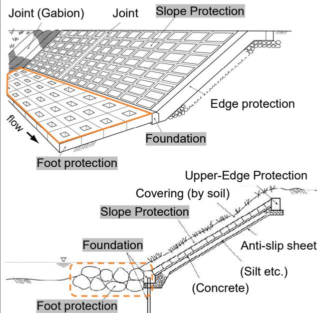
\*The most notable damage to bank protection is caused by **riverbed scouring** in front of it. In many cases, it is caused by **shallow Foundation**, or by **lack or washed-away of Foot protection**.
