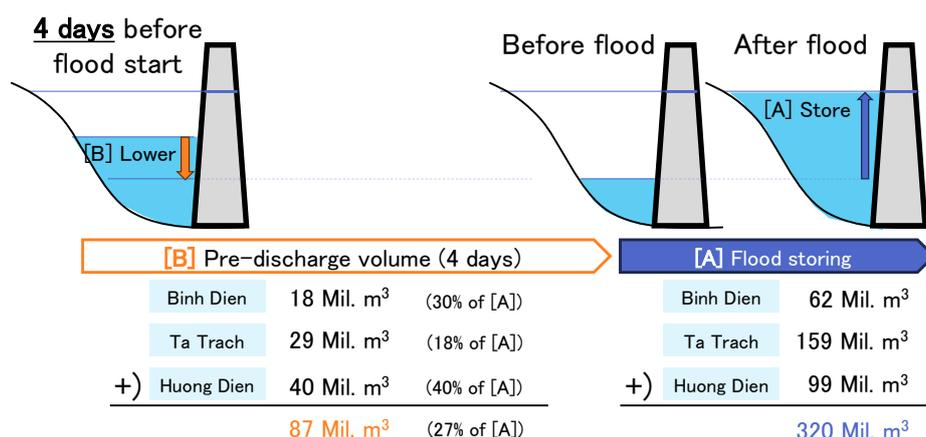
[Figure 6] Stored water volume [A] and the capacity secured by the prior lowering reservoir water level [B] in the three major dams
