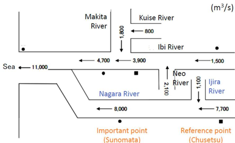
[Figure 4] Example of Discharge Diagram
