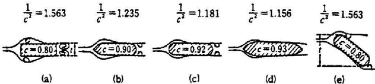
[Figure A.3] Constant  $C$ , determined by the plan shape of the pier for D'Aubuisson Formula.
