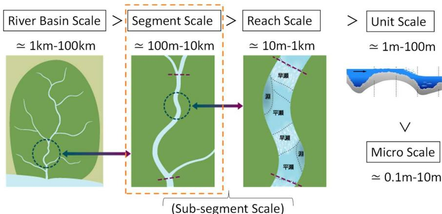
[Figure 2] Scales, hierarchical structure of rivers (b)
