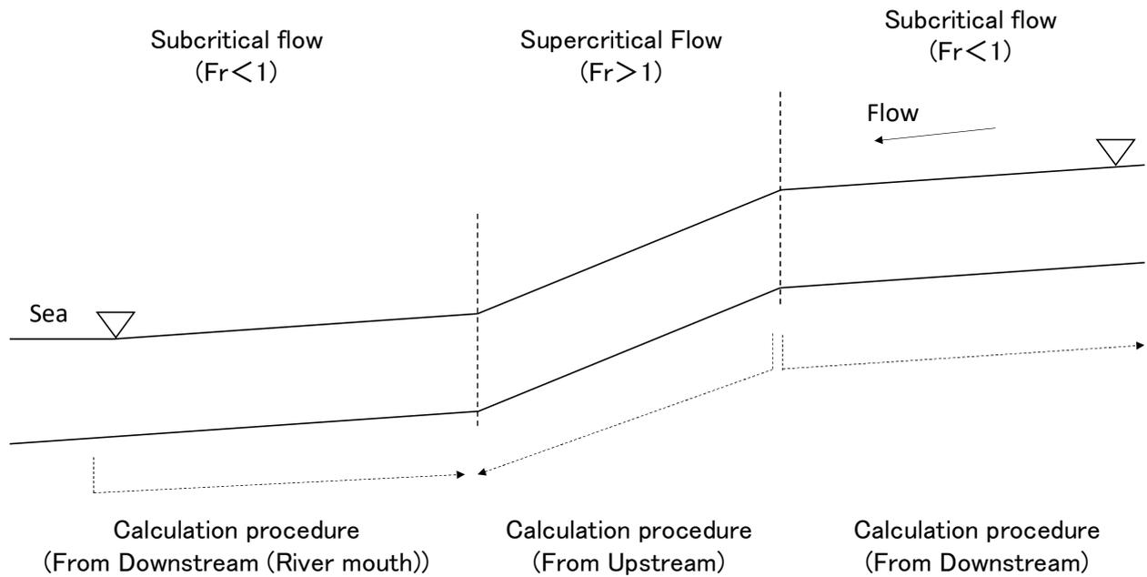
[Figure A.1] Calculation procedure when both subcritical flow section(s) and supercritical flow section(s) exist
